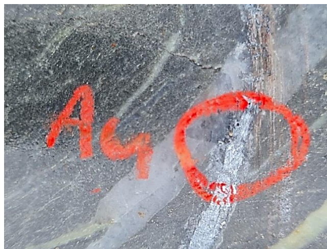
Figure 2: Coarse grained visible gold in stibnite vein (ELG152) in RVR's drilling at Eleanora-Garibaldi
