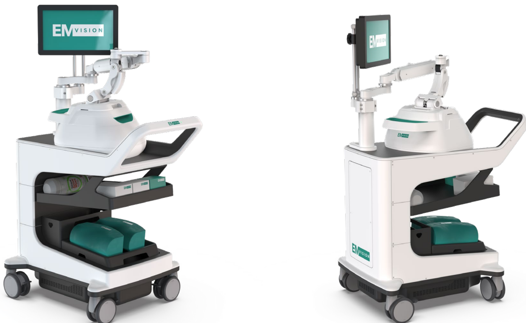
The above CAD images show the 1 st gen device, including headset, positioning arm and cart.
