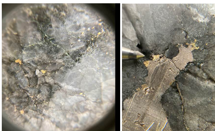
Photographs taken through a hand lens showing visible gold.
