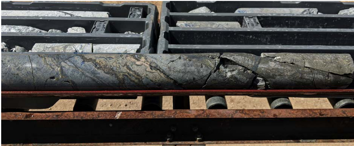
Figure 7: BD20012 from 230 to 234 metres, colloform sulphide and pebble breccia in the Northwest High-grade Zone.
