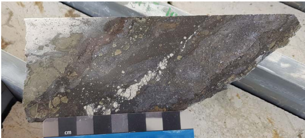
Figure 4. 128.1 metres in BD21002 (Main Zone) - Northern Feeder vein, with 1 metre @ 1,490 g/t silver, 4.36% lead and 2.2% zinc. Includes massive sulphide of sphalerite, galena and silver sulphides.
