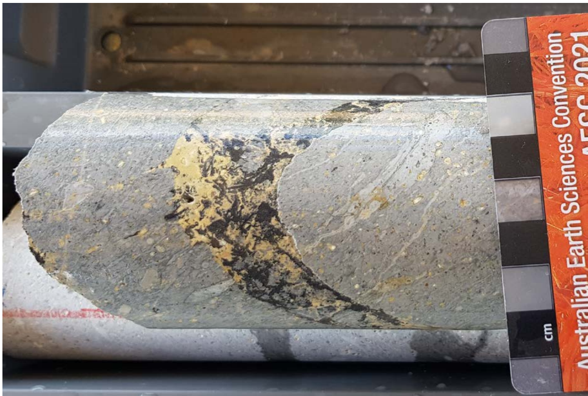
Figure 2: Coarse acanthite (silver sulphide) and carbonate vein in the Aegean Zone from BD21003 at 313 metres.
