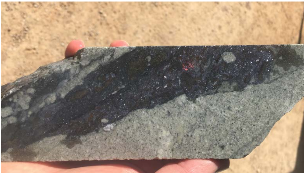
Figure 5. 279.4 metres in BD21001 - Northern Feeder vein, with 1 metre @ 1,290 g/t silver, 4.10% lead and 2.06% zinc. Includes massive sulphide of sphalerite, galena and silver sulphides.
