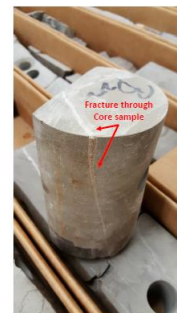
7217 – Vertical, filled fractures seen cutting through core.
