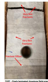
7229 - Finely laminated, limestone (light gray) / Shale (dark gray) interbedding. Very fine micro-fracture sets are seen throughout sample. Shale likely contains some organic matter.
