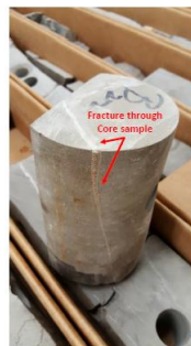
7217 - Vertical, filled fracture seen cutting through core.
