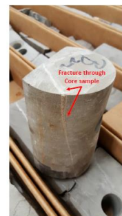
7217 - Vertical, filled fracture seen cutting through core.
