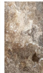
7210 - Large calcite crystals from fracture face. Some intercrystalline porosity.
