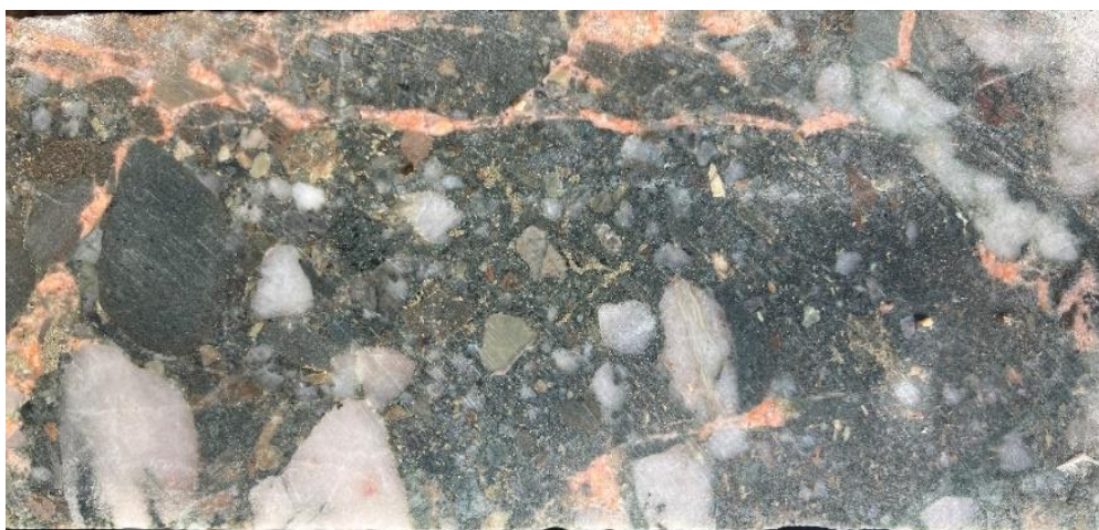
Figure 6: FI2079 core photo at 341.0m. Pink Kspar-quartz-carbonate infill irregular veins (<5mm). Associated fracture controlled pyrite with very minor chalcopyrite. The K-Spar vein indicates a Cu-rich hydrothermal event likely occurs in the Siluro- Devonian and this hole might be proximal to a copper zone. (NB: Assay, 1000 ppm Cu between 304 – 305m). Vertical width of photo is ~60mm.
