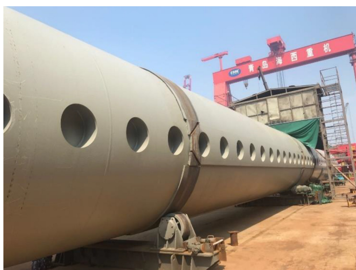
Platform legs completed and ready for connection
