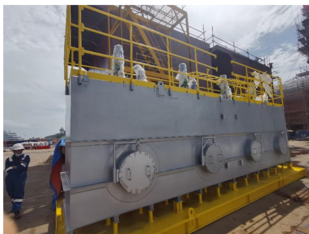
Production skid completed and ready for installation on the platform
