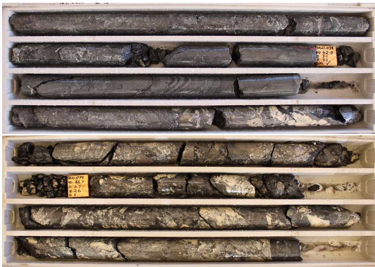
Figure 8: Drill hole SK21_039 showing Vein No.4 mineralisation intersected from 42.8m
