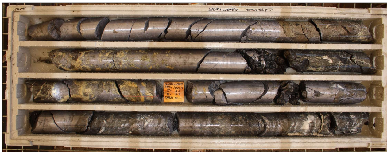
Figure 6: Drill core from hole SK21_027 massive galena showing part of the intersection of 9.5m @ 45.5% Pb, 4.1% Zn, 425g/t Ag from 174.4m
