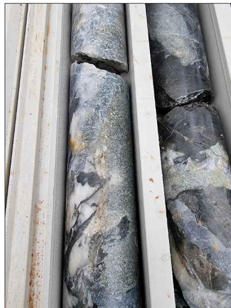
Figure 5: Quartz Tourmaline Chalcopryrite vein
