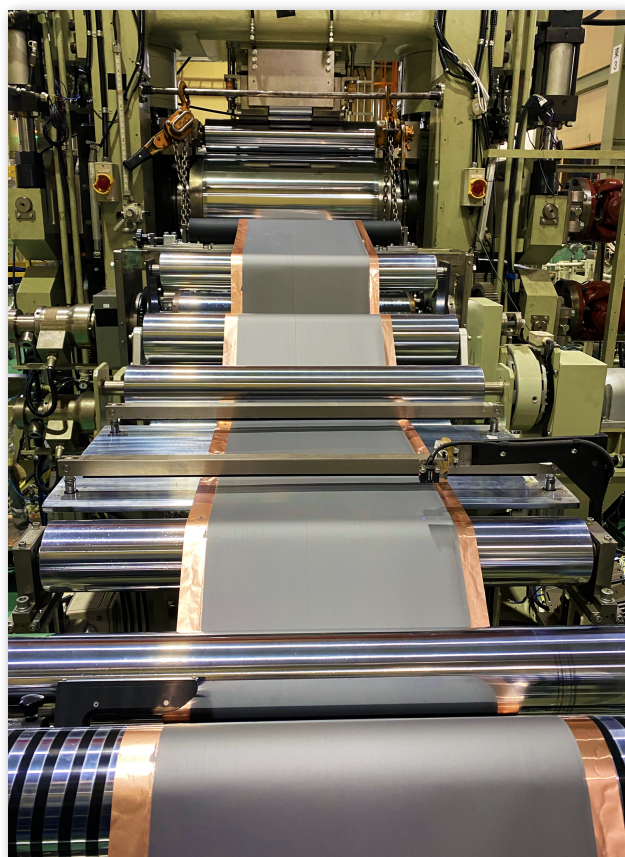
Figure 4 Talnode® coated onto current collector in automotive customer Li-ion battery cell pilot scale production.
