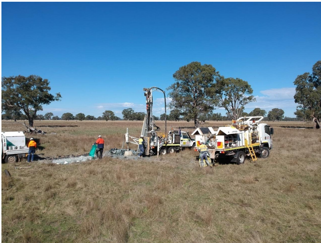
Photo 5. Air-core drilling at the Toora West prospect.
