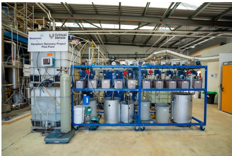
Figure 12 – Solvent Extraction section of Pilot Plant
