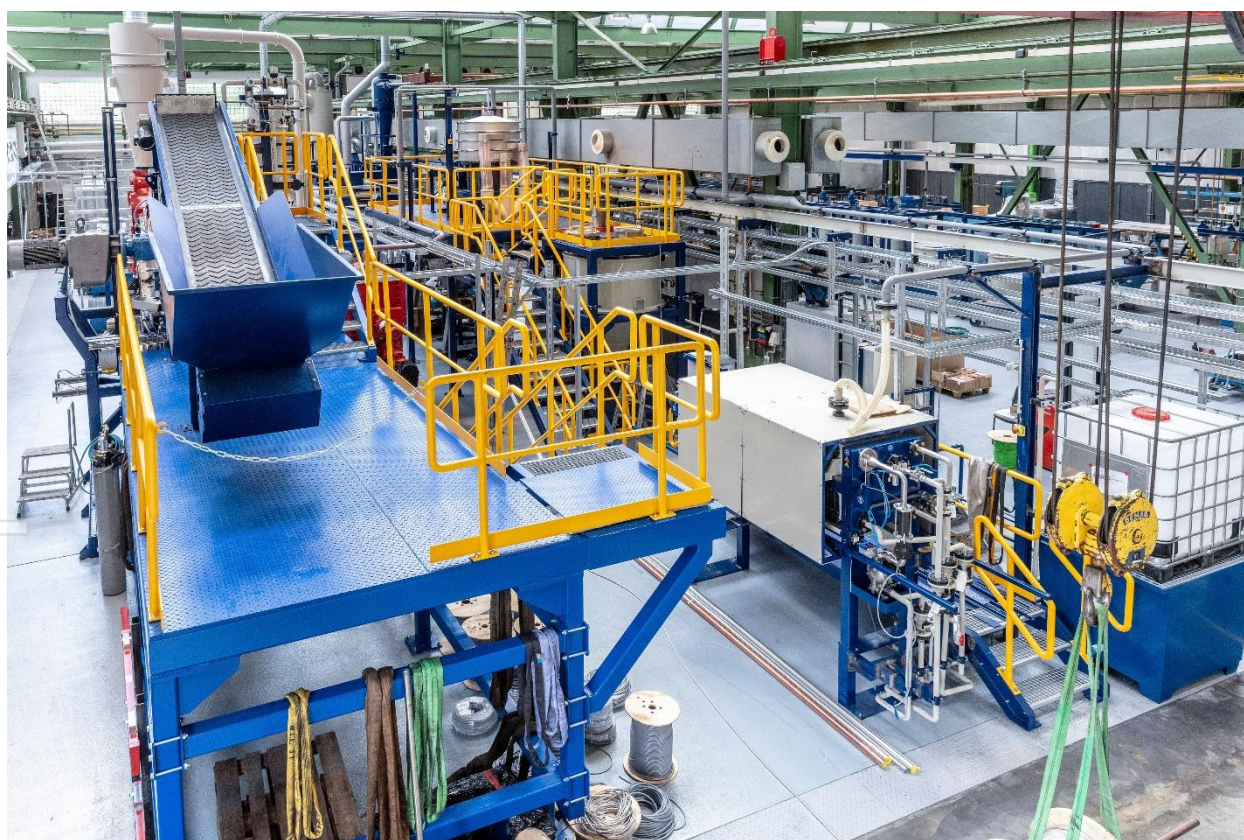
Figure 3 – Two stage Shredding Circuit
