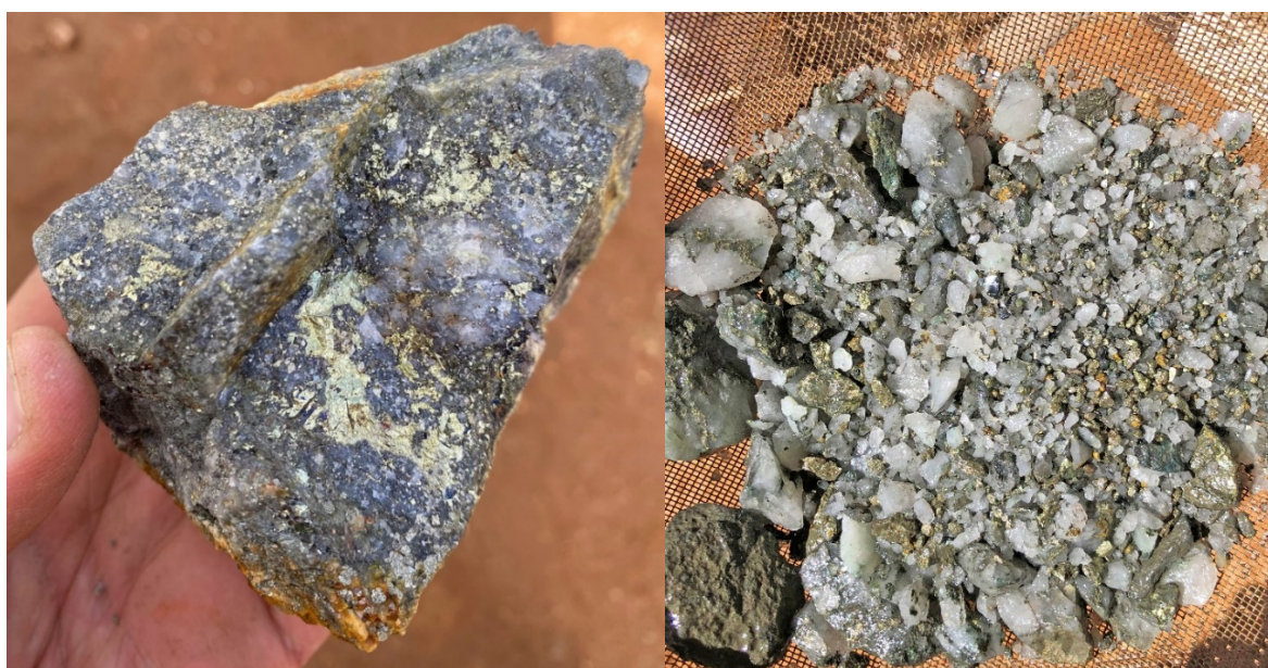
Figure 1. Comparison of quartz-sulphide mineralisation from Lake View surface dumps (left) with sieved chips from HMLVRC001, interval 44-45m assayed at 4.65% Cu and 0.52g/t Au (right)
