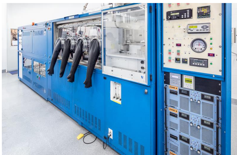
Pictured: A BluGlass RPCVD semiconductor wafer manufacturing platform, the BLG-300
