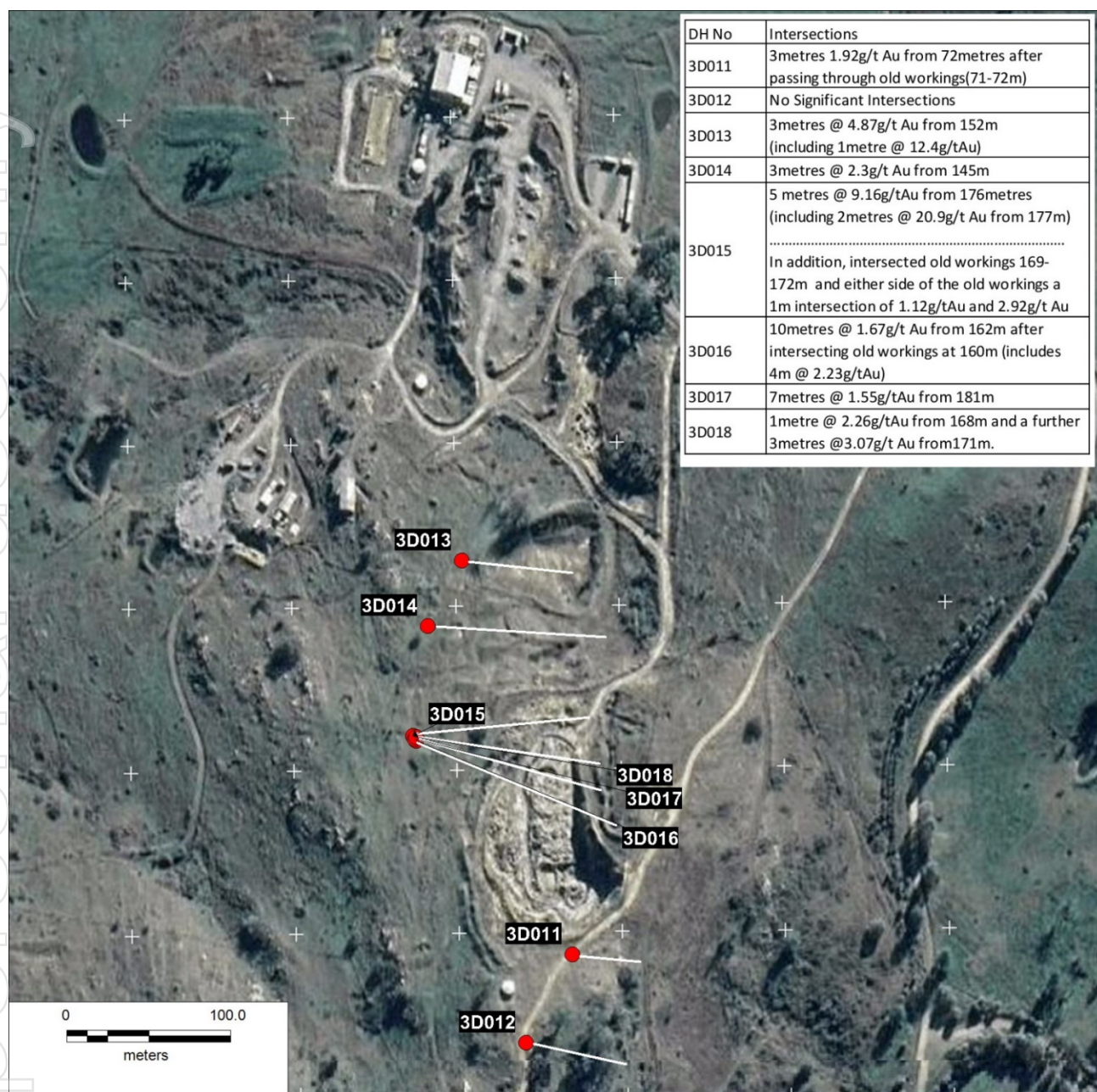
Figure 1: Drill Hole locations at Challenge deposit
