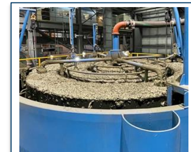
Additional cleaner column in operation and detailed design for Stackcell® completed. Expected to result in improved gold recoveries.
