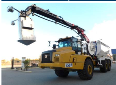
Robotic explosive placement
