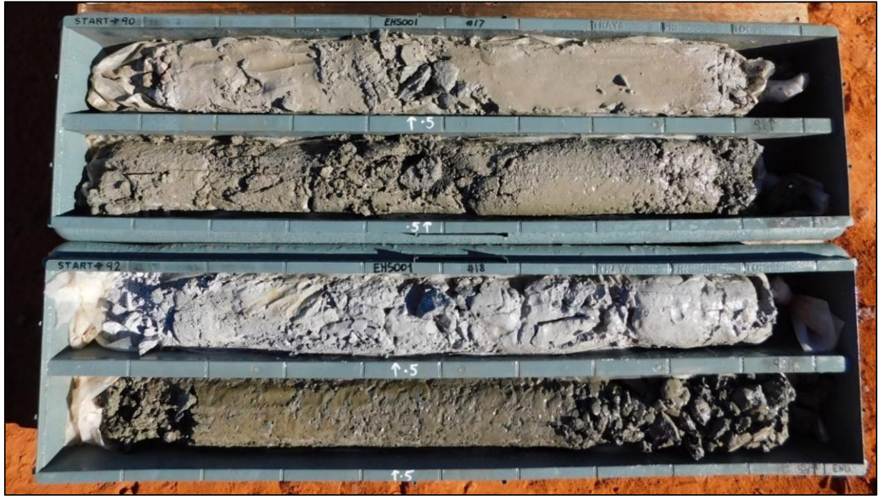
Image 2 – Mineralisation Zone –Sonic Drilling Core – EHS001 (twin of EHRC050). Sphalerite, galena and pyrite mineralisation was logged in this soft primary zone.
