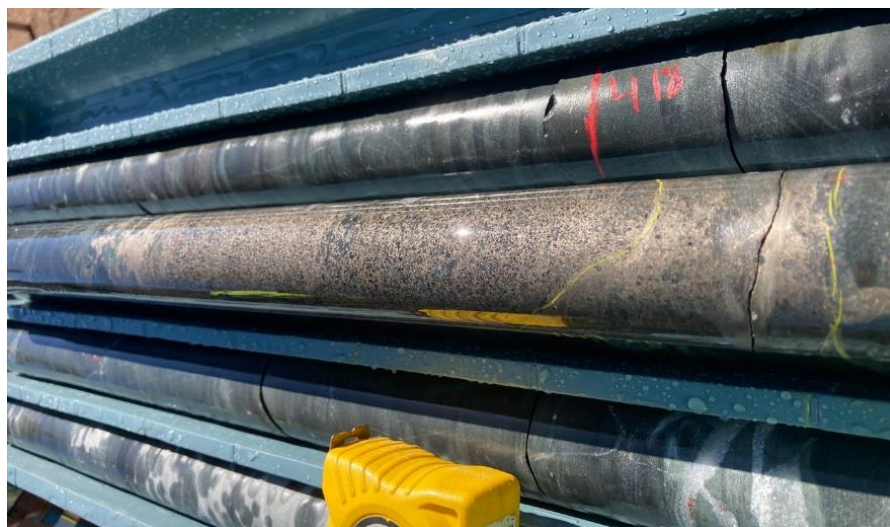
MDD371 intersection (0.8m @ 5.4% Ni) – massive and matrix sulphides
