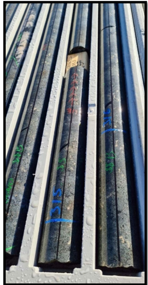
Photo 1: Ni-Cu sulphide mineralisation from RKDD065 from 314m
