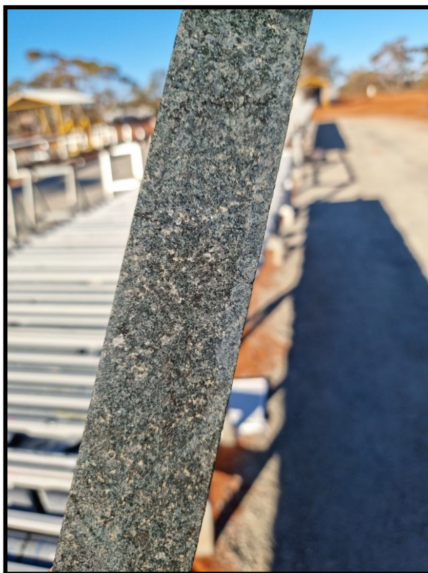
Photo 2: Disseminated Ni-Cu sulphide from RKDD064 from 304m
