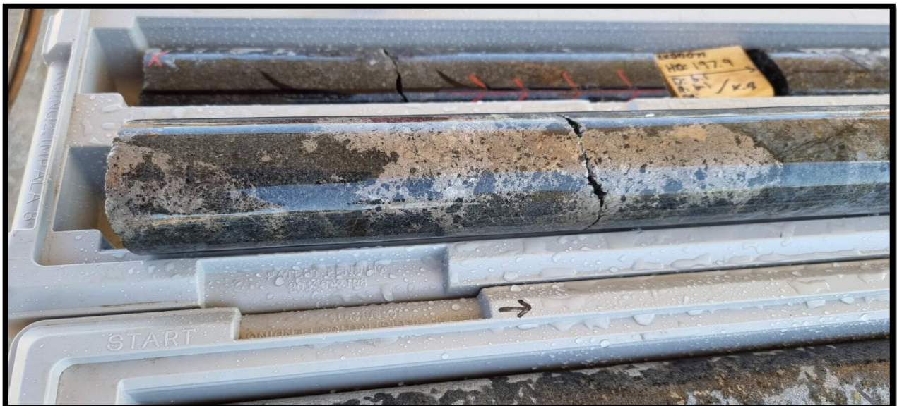
Photo 5: Ni-Cu sulphide mineralisation from RKDD71 from 201m
