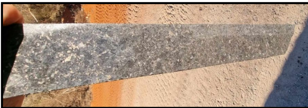
Photo 4: Ni-Cu sulphide mineralisation from RKDD066 from 266m
