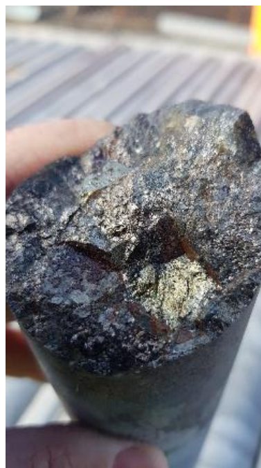
Image 3 – MDRCD 375 – coarse grained pyrrhotite +/- pyrite
