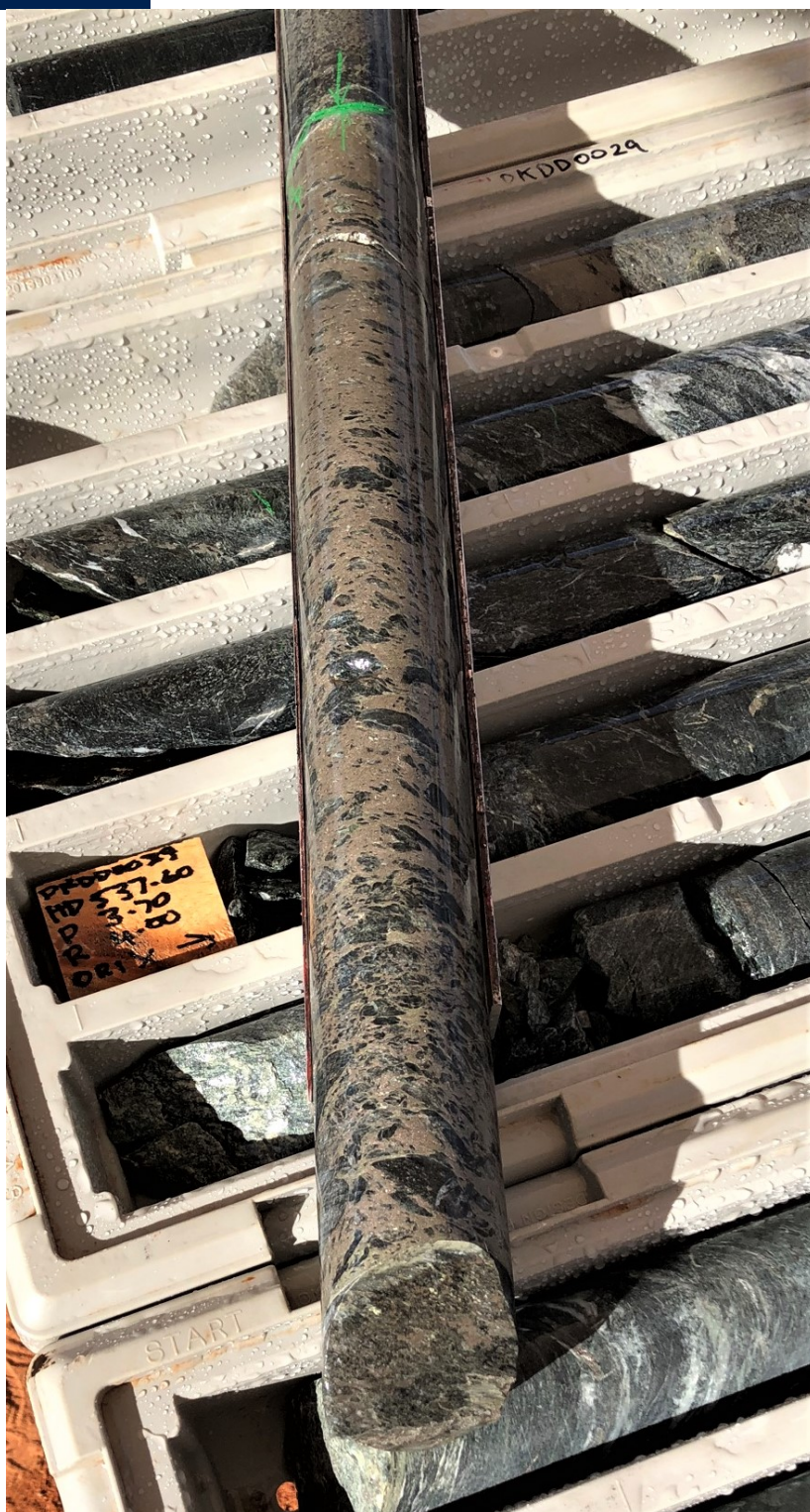
Figure 2: A close-up of the intersection of massive sulphide in DKDD0029
