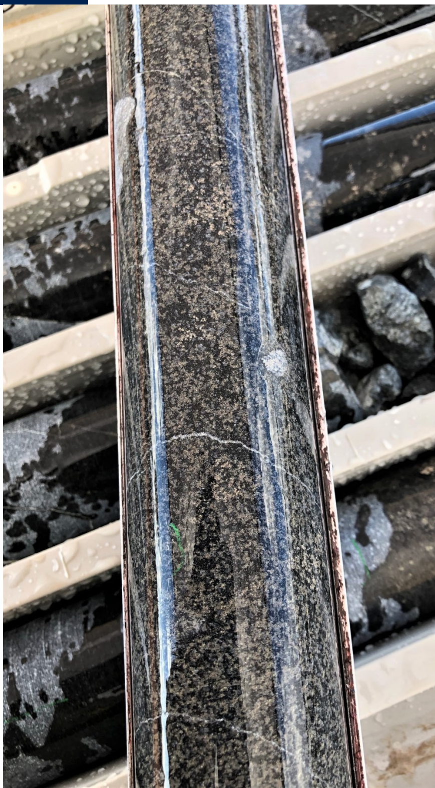
Figure 3: Heavy disseminated sulphides in drillhole DKDD0029
