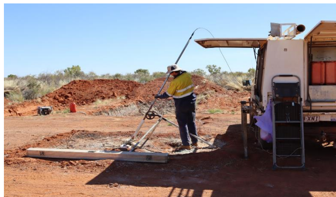
Figure 4: GAP Technician sending the DHEM probe down hole NR108D026
