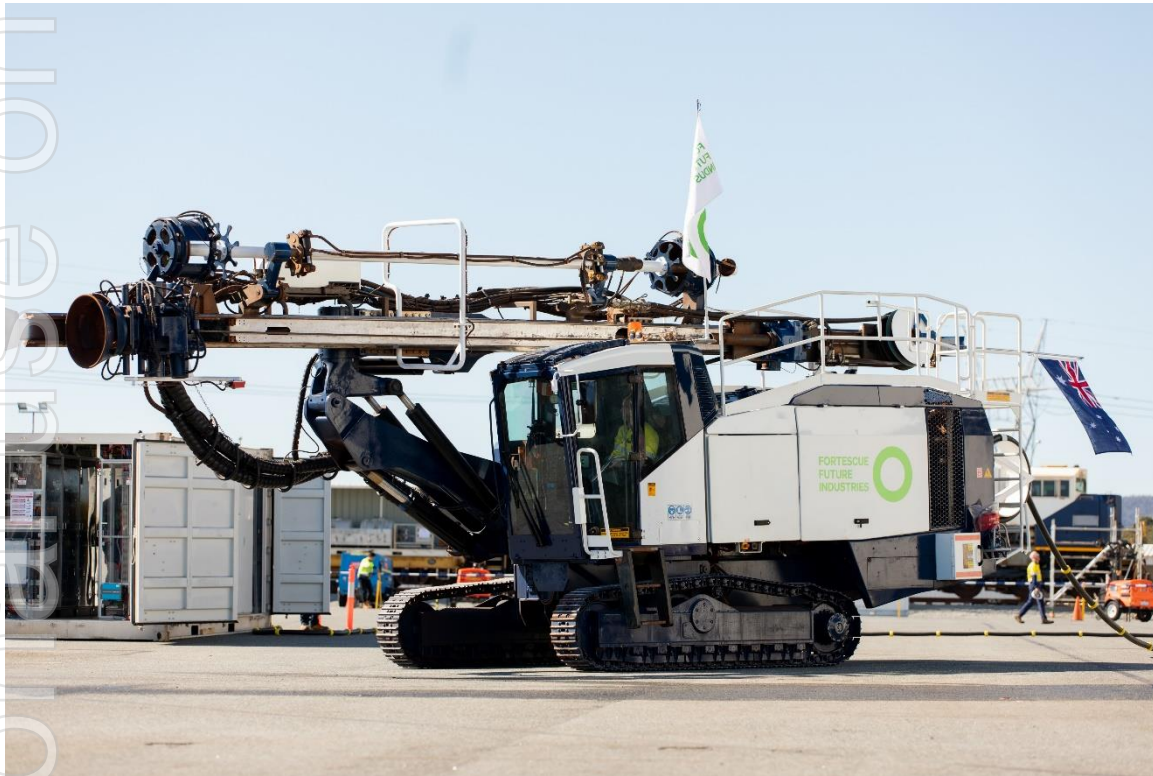
Systems testing on hydrogen powered drill rig for technology demonstration
