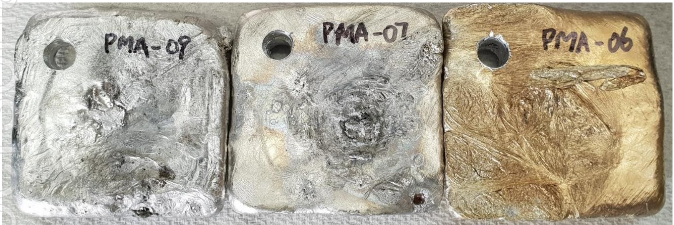
Figure 2: Master alloys produced from three different scandium chemicals from intermediate stages within the PSP scandium recovery flowsheet.
