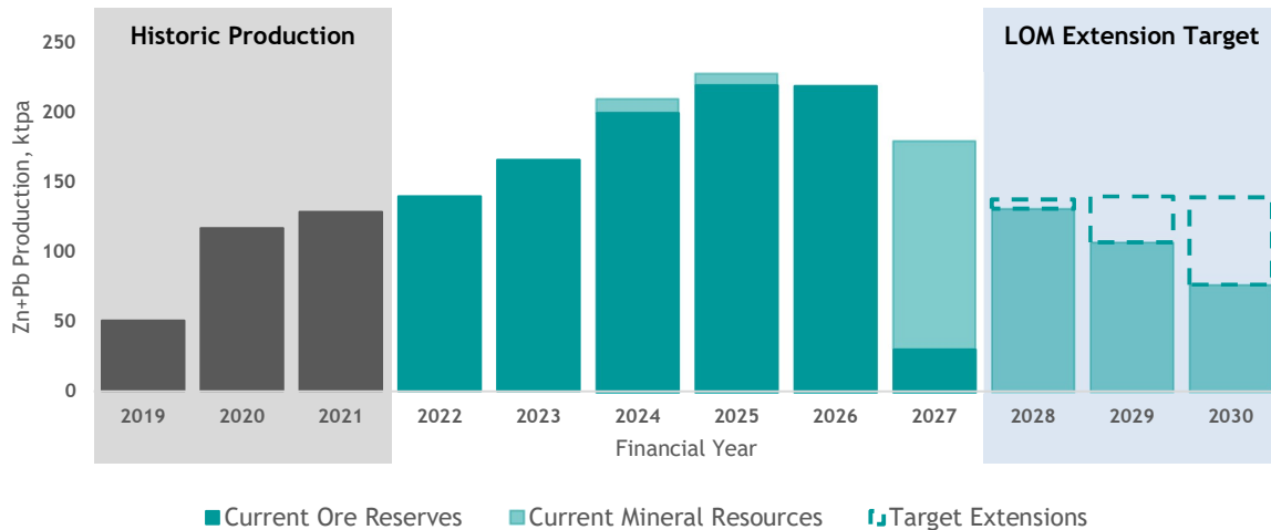
Figure 17: Mined ore production profile showing potential mine life extension with the inclusion of Silver King Resource, South Block and Watson's Lode and a target extension to current resources
