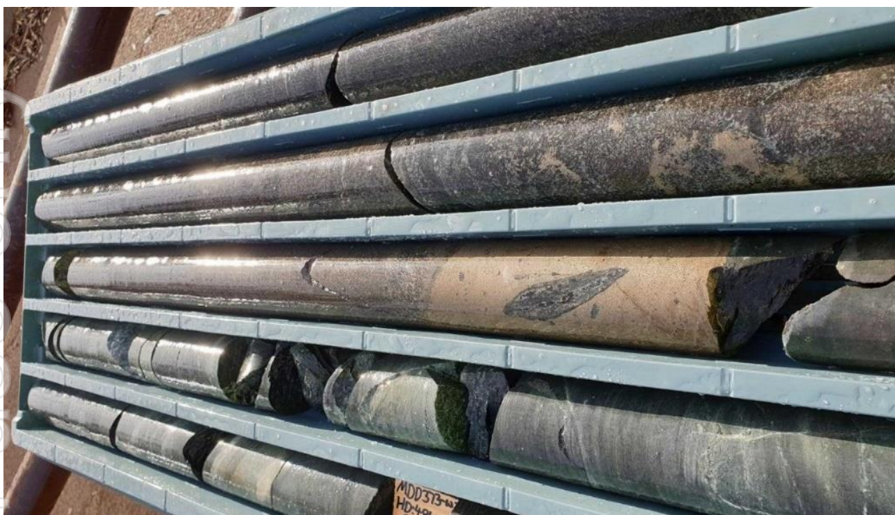
MDD373W2 intersection (4.5m @ 3.3% Ni) – massive and matrix sulphides core, prior to assays
