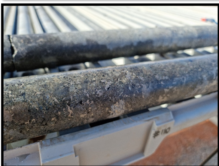
Photo 2: Sulphide mineralisation from OCDD001 (clockwise) from 541.6m, 579.5m, 545.0m, and 603.0m downhole.
