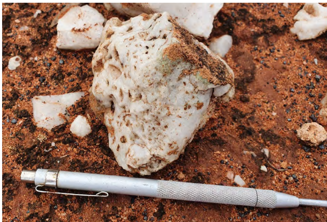
Figure 8-2: Quartz float showing marks (after-sulphides)
