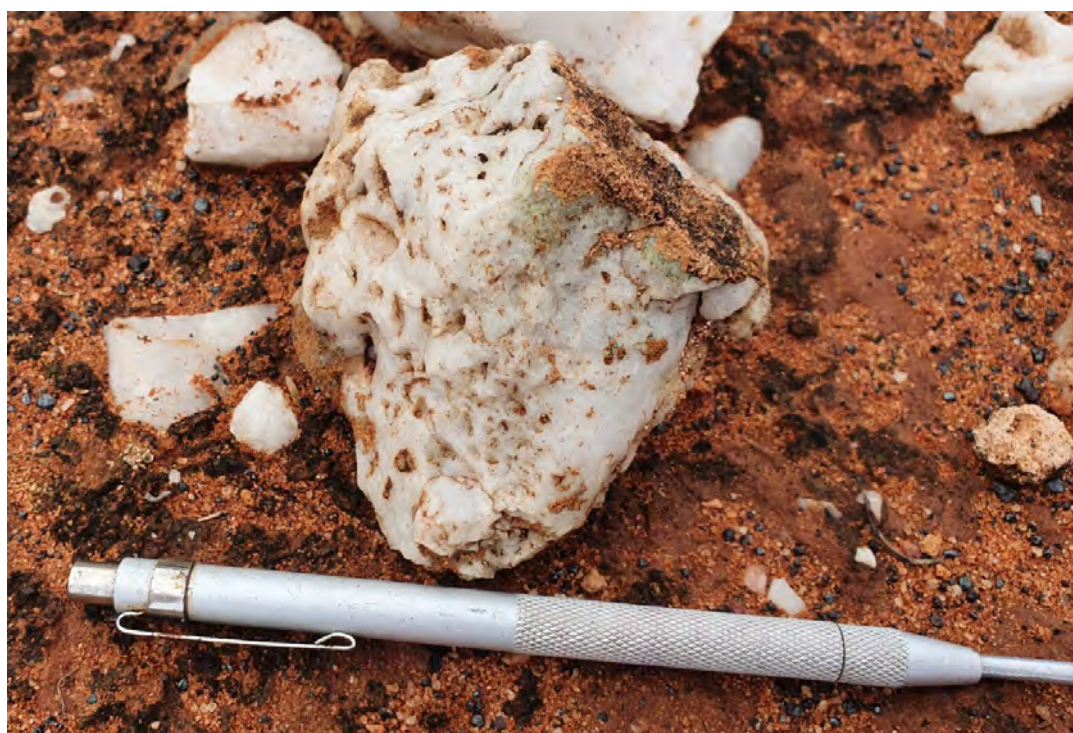
Figure 8-2: Quartz float showing marks (after-sulphides)
