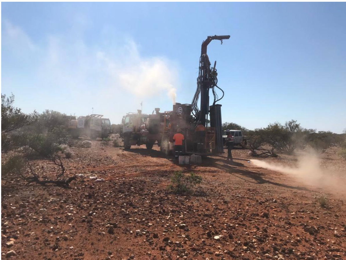
Figure 1: Aircore Drilling Rig at the Shadow Prospect of the Austin Gold Project.
