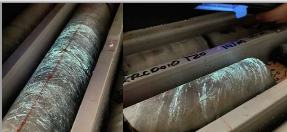
Figure 7: Bornite (copper sulphide) with malayaite (calcium-tin-silicate) fluorescing under UV light in 3KRC010. Drillcore is 61.1mm wide for scale.
