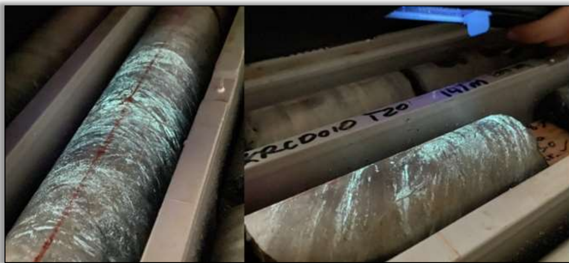
Figure 7: Bornite (copper sulphide) with malayaite (calcium-tin-silicate) fluorescing under UV light in 3KRCDD10. Drillcore is 61.1mm wide for scale.
