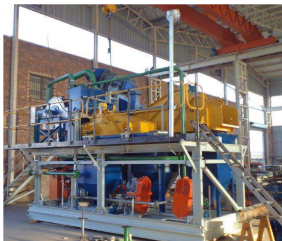
Figure 5 – Example of the the dense media separation unit to form part of the extraction plant
