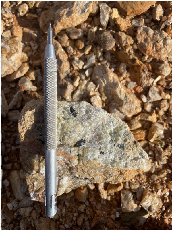
Figure 3: LHS shows quartz rich portion of a pegmatite showing very coarse grained cassiterite (555380mE and 6531663mN).
