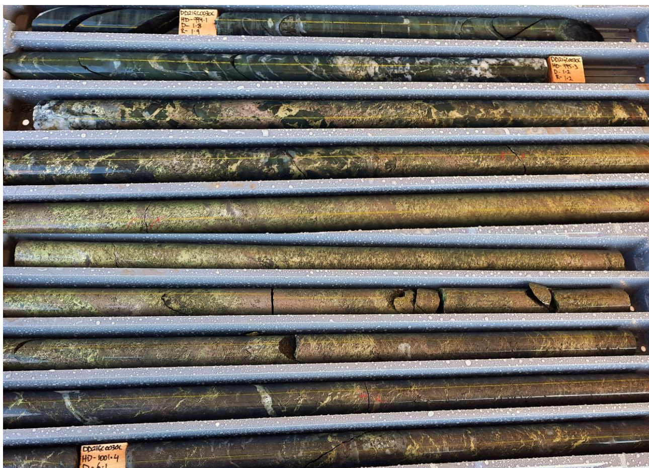
Figure 1. Composite image of drill core with high grade copper mineralisation from DD21GC0030C containing massive and semi-massive chalcopyrite (yellow) and pyrrhotite (light brown). A portion of the displayed core returned grades of 10.8% Cu, 1.2g/t Au & 31g/t Ag over 4.7 metres.
