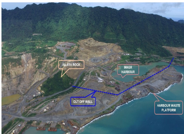
Figure 6 & 7 – Cut of wall Alignment and Seepage Barrier / Kapit Pit at EOM
