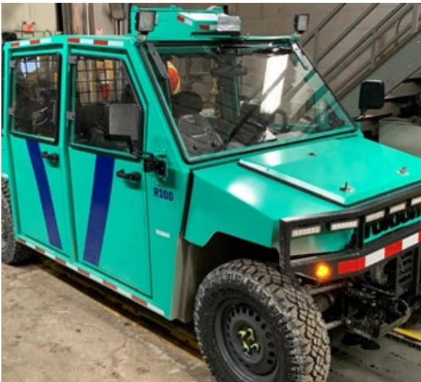
Rokion R100 battery electrical vehicle (BEV) for underground at Red Lake
