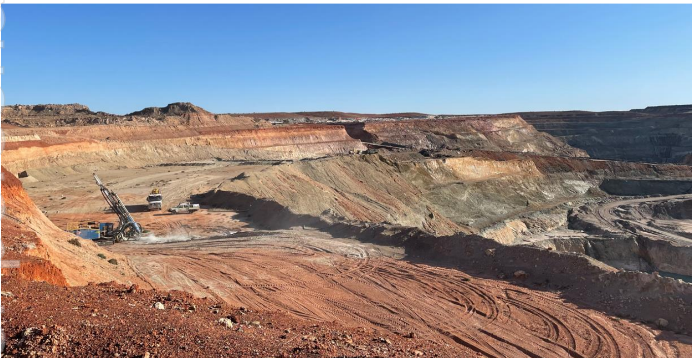
Figure 3: Commencement of grade control drilling in the KOTH southern pit.
