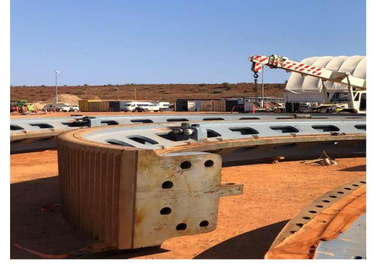
Assembly of girth gear for 36-foot diameter SAG Mill
