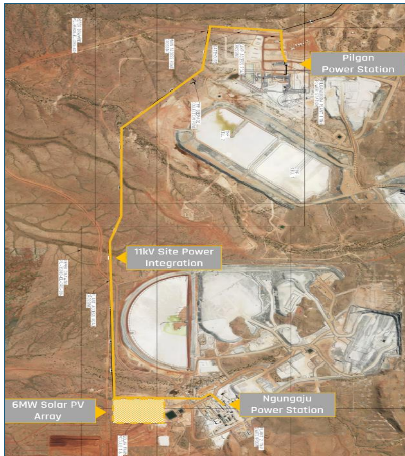
Figure 1 – Proposed Location of the 6MW Solar Array and power integration at Pilgangoora
