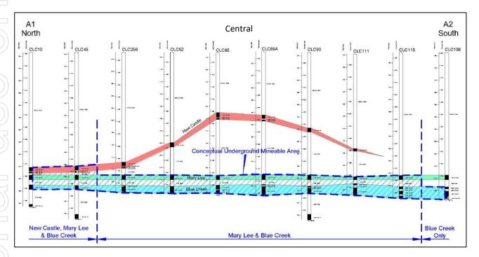
The above cross section illustrates the coal seam stratigraphy noting in particular;
