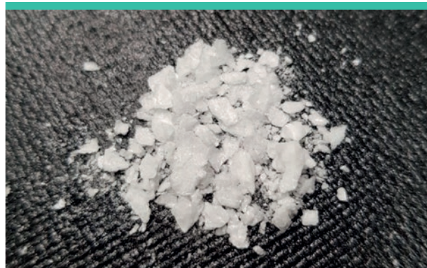
High purity (99.995%), lithium-ion cathode pre-cursor
