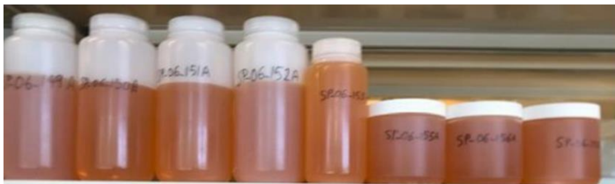
Figure 5 – ASX 22/09/21: Solution of Supplied Kaolin after Digestion
