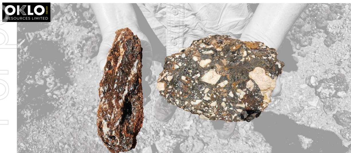
Figure 1: Bembala North - sample of a sheared breccia (left) showing similarities to SK1.
