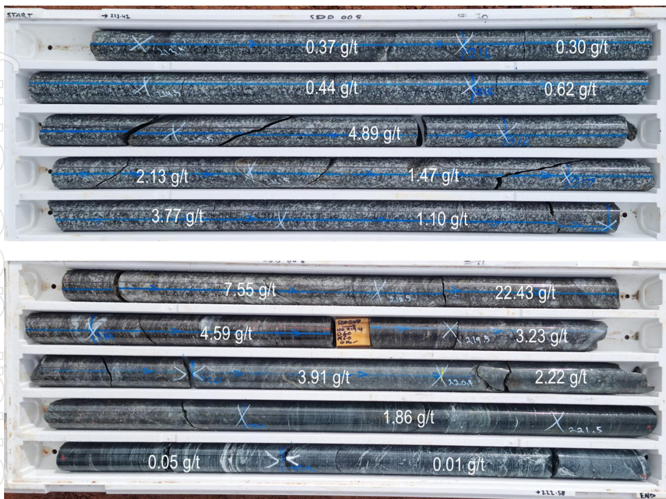
Figure 9: (SDD008) -Lord Nelson NQ (47.6mm) diamond core from 213.42m to 222.58m showing high-grade gold mineralisation in strong quartz-pyrite veining, along the contact between silicified granodiorite and strong foliated ultramafic contact
