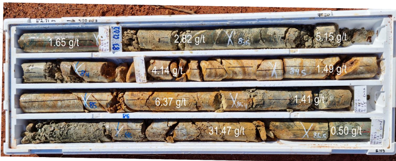
Figure 7: (SDD003) -Orion Lode HQ (63.5mm) diamond core from 82.71m to 86.7m showing high-grade gold mineralisation in oxide and transitional zone.
