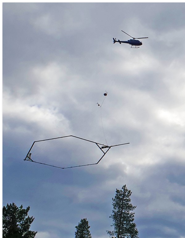
Figure 1 SkyTEM system airborne on Talga project.
