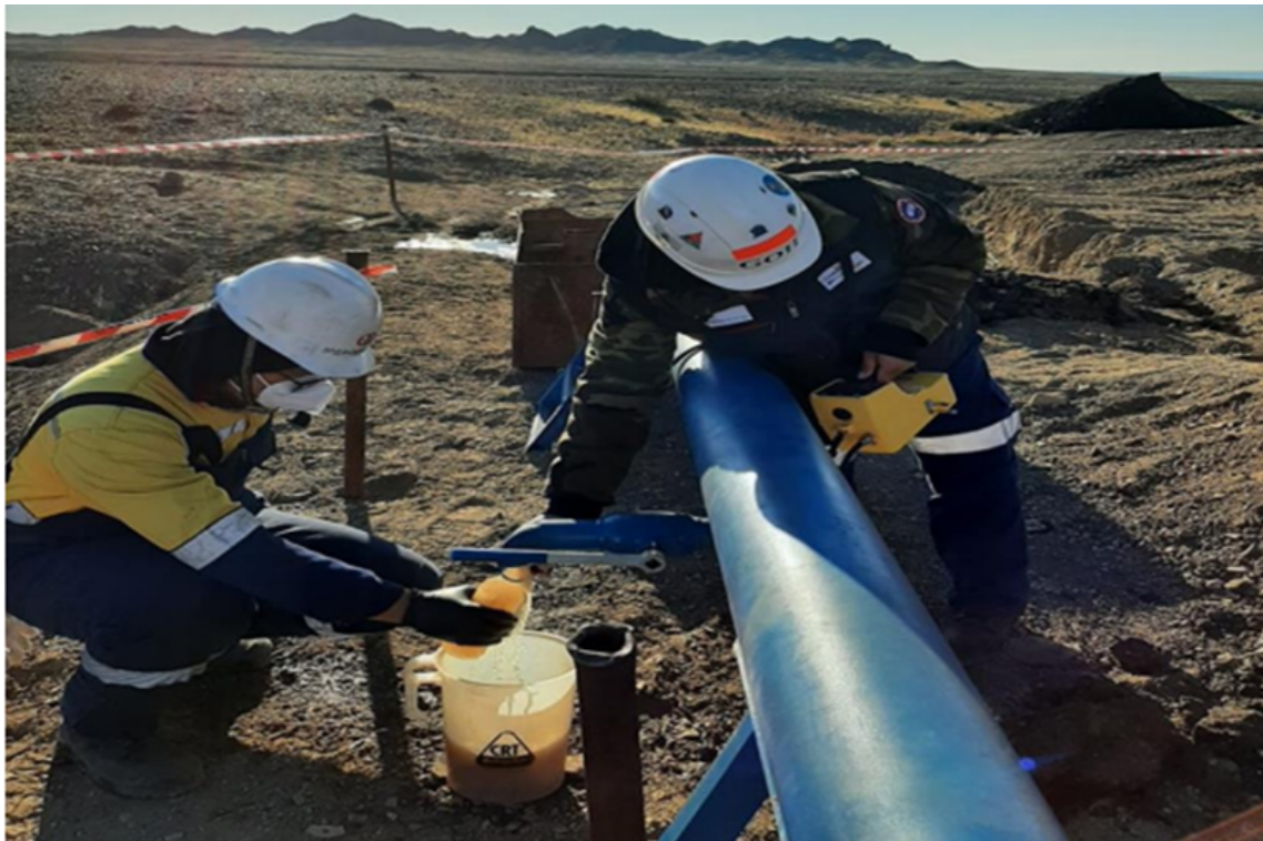
Gas testing and water sample gathering at Nomgon 6
