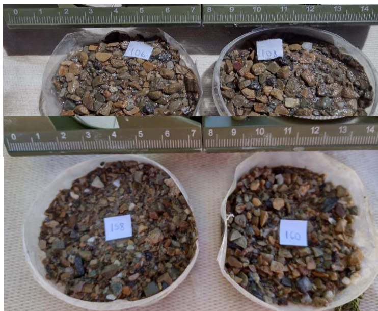
Figure 2: Cuttings of drill hole PB-01-21. These are cuttings of a polymictic conglomerate which we now know to extend through a min 40m zone of no recovery from the previous adjacent drill
