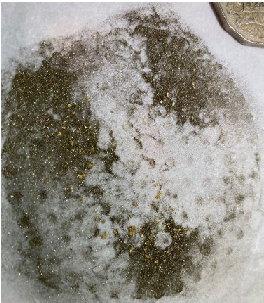
Plate 1 – Gravity gold concentrate obtained from a 5kg – 15g/t Au transitional basalt sample rod milled to P 80 passing 75 micron then gravity concentrated – via Knelson centrifugal concentrator (phase 1) and the Mozley Table (phase 2); large nuggety gold grains visible in concentrate. Larger grains flattened due to rod milling process.
