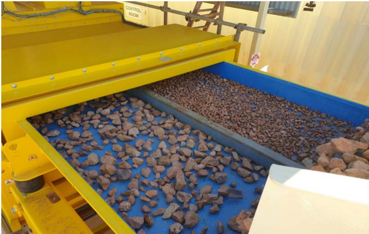
Figure 3: Feeder with simultaneous feed of two size fractions of ore to the ore sorter machine
