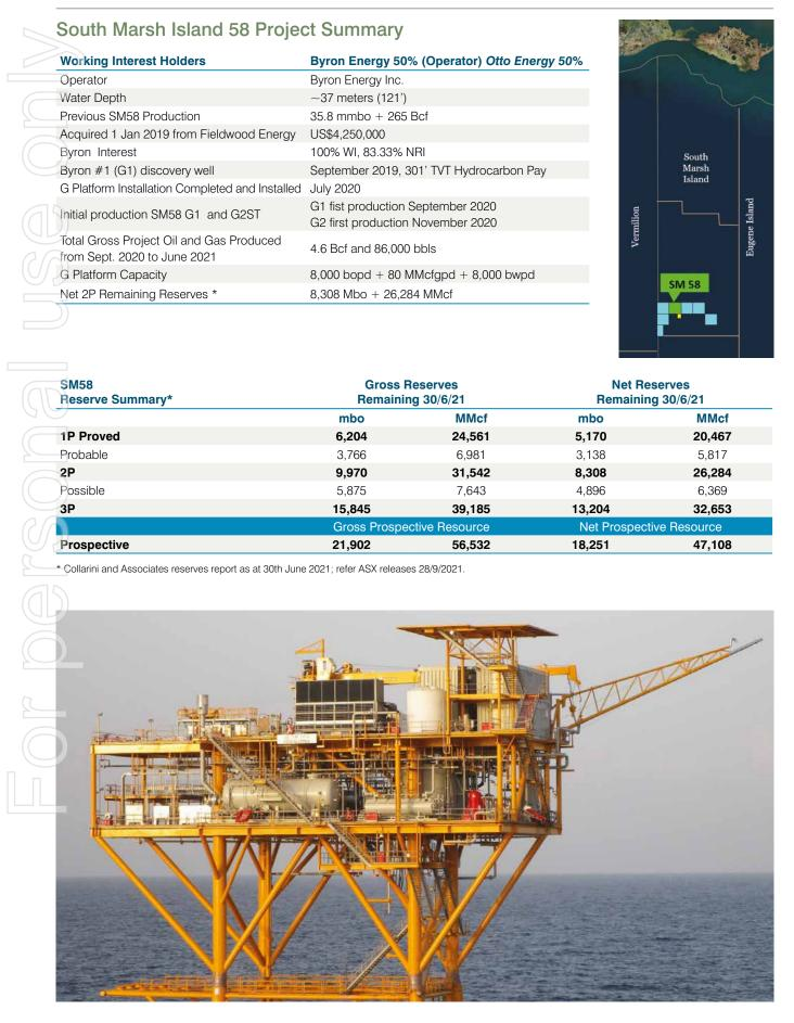
The SM58 G2ST well was tied into the SM58 G platform and the O Sand was opened to production on 29 October 2020 and has now produced approximately 0.64 Bcfg and 42,000 barrels of oil with an estimated 9,600 barrels of formation water.
