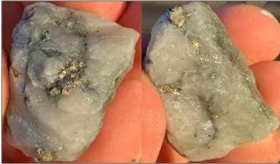
Mineralised quartz veins at 334.9m – Graded at 1.22g/t Au
